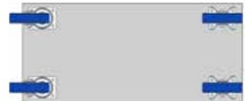
Two swivel and fixed castors with identical mounting height
