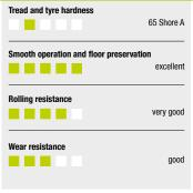
To make it easier for you to choose the correct product, we provide a Blickle info box for each wheel series on the relevant page. This provides an overview of the tread and tyre hardness of a wheel, its smooth operation and floor preservation, rolling resistance and wear resistance.
